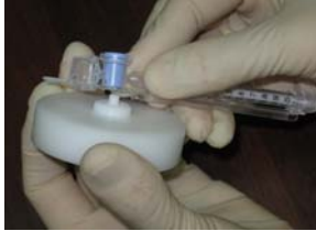
Reposition the blue valve with the jig
