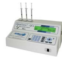
Figure 4: On-board heating unit pre-heats 3 testing capillaries and 3 collection cups
