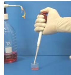
Figure 3: Add sample to pre-heated diluent
