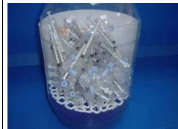
Capillaries drying on plastic net above silica beads
